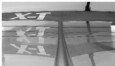
Correct batten tension
