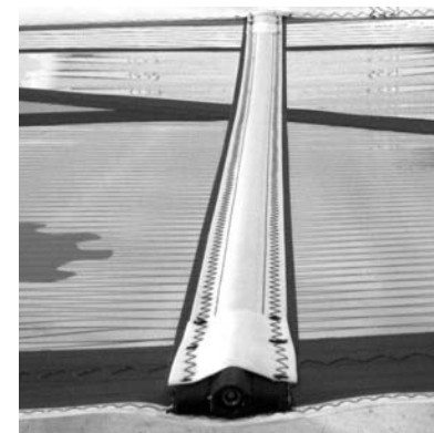
▲ needs batten tension
