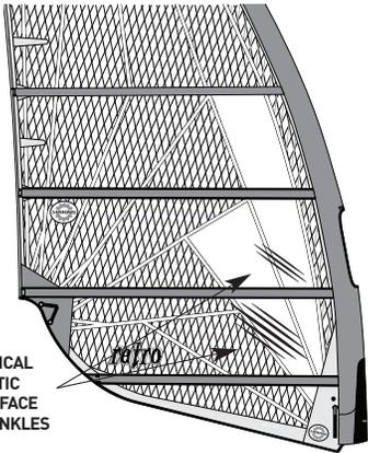
**A** The Retro has some diagonal wrinkles in the foot area that are visible when the sail is static (unloaded). They are associated with the flexible nature of a semi-rigid three-dimension structure and are not indicative of a construction problem or error. They are a by-product of the very deep broadseaming profile and elastic rotation of the foil from static to loaded forms.
