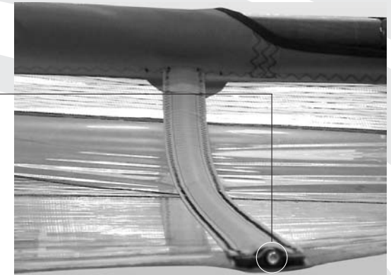
▲ needs batten tension ▼ perfect batten tension
