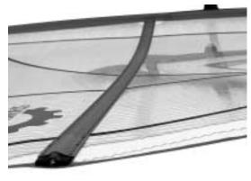
a smooth reflection, with no wrinkles alongside the battens. Batten tension should be tightest on the lower battens and looser on the upper battens.
