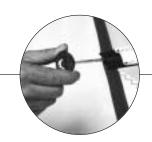
The battens are tensioned using the hex-key tool found under the Velcro tab above the tack handle. Insert the hex-key into the cap screw inside the end of each SBT at the leech end of each batten. Turn the hex-key to the right (clockwise) to tighten. Tension the battens JUST until the small wrinkles across the batten pockets disappear. Look for continuous smooth shape to the sailcloth adjacent to the batten pocket (see photos). You should see
