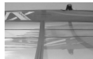
Needs more batten tension
