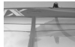
Correct batten tension
