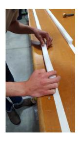
The shorter 8" piece of elastic requires lacing onto the tri-glide fasteners, then elastic parts were then sewn. One end of the shorter (8") elastic is bar-tacked to the center bar of the tri-glide fastener with as short a tail as possible. One end of the longer (12") elastic is folded and bar-tacked to itself to form a 1/2" stopper end. We ganged up long runs of the parts and bar tacked them on automatic Juki LU-2828 sewing machines with a 5-stitch x 5 pass stitch pattern.
