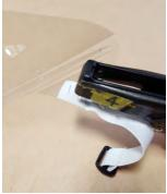
Some background here, as stapling the elastic to the PET film was a hot point of discussion and testing in our development of the face shield construction. It's not a very high tech or elegant solution, but it proved be the best choice for a few reasons. First, its fast and easy, and imposes the least amount of handling on the PET film lens. It also proved to be quite strong for the purposes of the face shield. The alternatives we tested were sewing the elastic to the PET film, both
