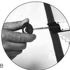
the leech end of each batten. Turn the hex-key to the right (clockwise) to tighten. Tension the battens JUST until the small wrinkles across the batten pockets disappear. Look for continuous smooth shape to the sailcloth adjacent to the batten pocket (see photos). You should see a smooth reflection, with no wrinkles alongside the battens. Batten tension should be tightest on the lower battens and looser on the upper battens.
