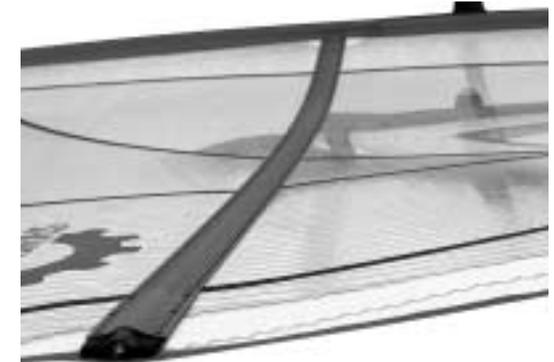
**CAUTION: DO NOT OVER-TENSION THE BATTENS – POOR ROTATION, EXCESSIVE FOIL DEPTH AND DAMAGE TO THE SAIL CAN RESULT.**
