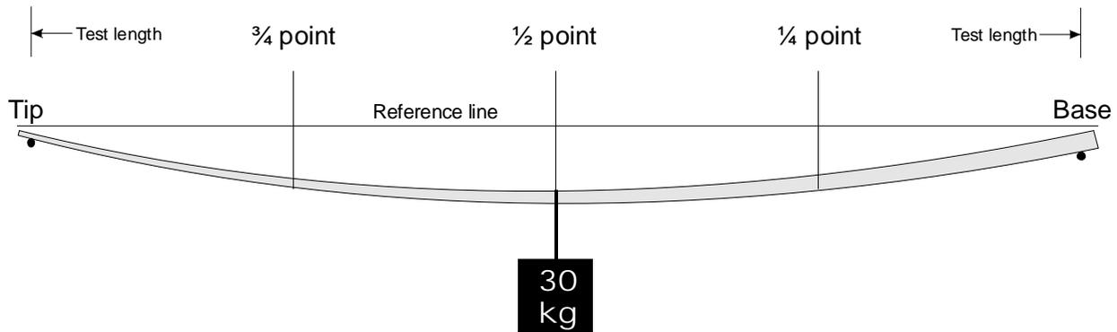
8. Tabulate the results by subtracting the pre-bend from the loaded bend at each point. This is the net deflection for each point.
